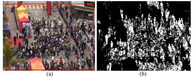
Fig. 1. (a) Typical scene to be processed. (b) Binary foreground image after background subtraction for (a).
