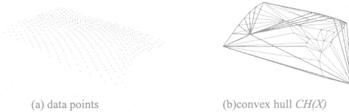
Figure 4 Computing convex hull of data points with increment method
