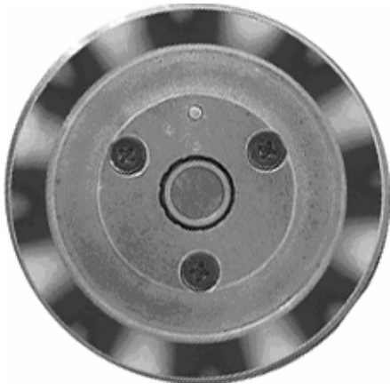
Figure 10. Measured vibration pattern using laser Doppler vibrometer.
