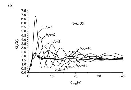
**Fig. 4.** Normalized dynamic energy release rates for various width's piezoelectric strips as  $h_2/h_1=1$  with normalized time under shear impact, PZT-4/BaTiO<sub>3</sub>, a/c=1: (a) electric impermeable cracks; (b) electric permeable cracks
