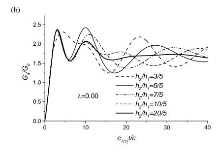
**Fig. 5.** Normalized dynamic energy release rates for various ratios of  $h_2/h_1$  as  $h_1/c=5$  with normalized time under shear impact, PZT-4/BaTiO<sub>3</sub>, a/c=1: (a) electric impermeable cracks; (b) electric permeable cracks
