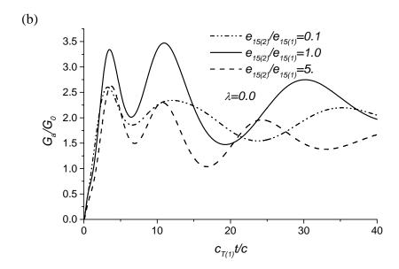
**Fig. 8.** Normalized dynamic energy release rates for various ratios of piezoelectric constants with normalized time under shear impact, a/c=1,  $h_2/h_1=1$ ,  $h_1/c=5$ : (a) electric impermeable cracks; (b) electric permeable cracks
