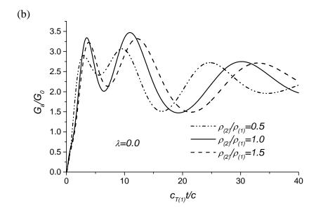
**Fig. 10.** Normalized dynamic energy release rates for various ratios of material densities with normalized time under shear impact, a/c=1,  $h_2/h_1=1$ ,  $h_1/c=5$ : (a) electric impermeable cracks; (b) electric permeable cracks
