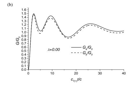
**Fig. 2.** Normalized dynamic stress intensity factors and energy release rates at x=a and x=b with normalized time for electric impermeable interface cracks under shear impact, PZT-4/BaTiO<sub>3</sub>, a/c=1,  $h_2/h_1=1$ ,  $h_1/c=5$
