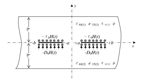
**Fig. 1.** Two dissimilar piezoelectric strips with two coplanar interface cracks under anti-plane mechanical impact and electrical impact
