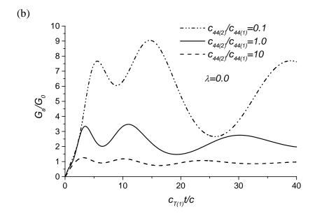
**Fig. 7.** Normalized dynamic energy release rates for various ratios of elastic constants with normalized time under shear impact, a/c=1,  $h_2/h_1=1$ ,  $h_1/c=5$ : (a) electric impermeable cracks; (b) electric permeable cracks
