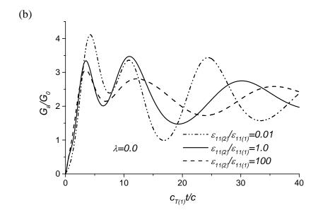
**Fig. 9.** Normalized dynamic energy release rates for various ratios of dielectric constants with normalized time under shear impact, a/c=1,  $h_2/h_1=1$ ,  $h_1/c=5$ : (a) electric impermeable cracks; (b) electric permeable cracks
