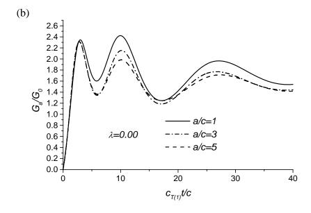
**Fig. 6.** Normalized dynamic energy release rates for different relative crack positions with normalized time under shear impact, PZT-4/BaTiO<sub>3</sub>,  $h_2/h_1=1$ ,  $h_1/c=5$ : (a) electric impermeable cracks; (b) electric permeable cracks
