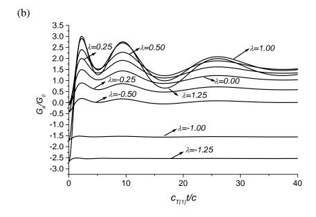
**Fig. 3.** Normalized dynamic stress intensity factors and energy release rates for various load combination parameters with normalized time for electric impermeable interface cracks, PZT-4/BaTiO<sub>3</sub>, a/c=1,  $h_2/h_1=1$ ,  $h_1/c=5$
