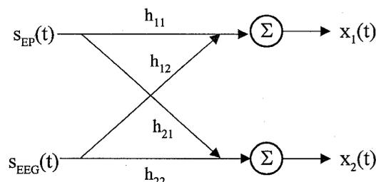
Fig.1 Model of two channel observations
