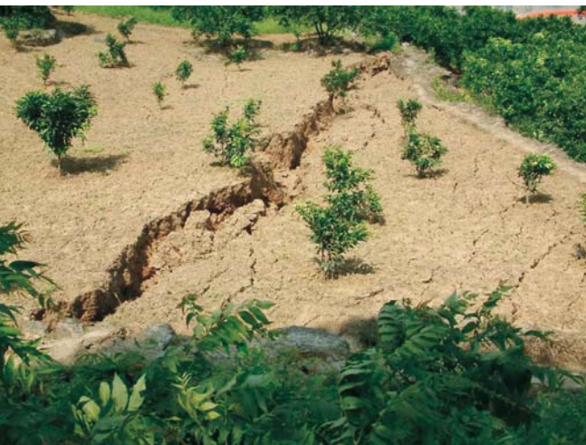
Fig. 9. A long fissure observed on the remaining slope on the left side of the landslide.
