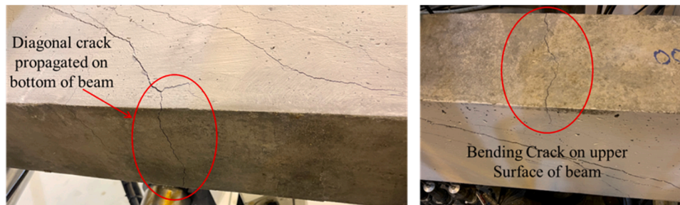
Fig. 7. Major cracks on the top and bottom surface of the REF-R100 beam specimen.
