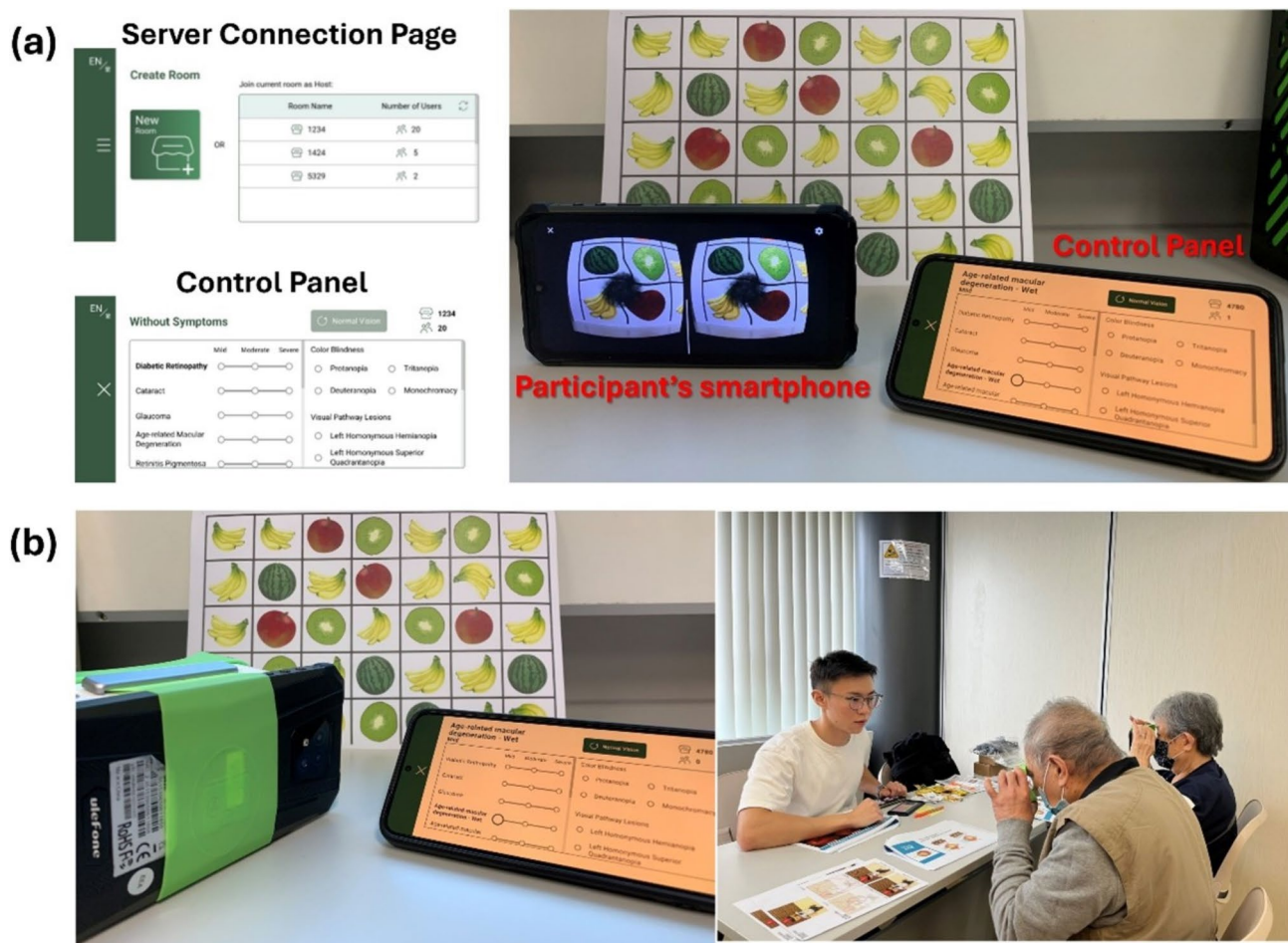
Fig. 2 Setup of the AR device. (a) A smartphone can be set up as the controller by creating a server using the mobile application interface. The participants' smartphones can then be connected to the created server, enabling the workshop instructor to apply simulated visual defects to their devices using the control panel interface. (b) The participants' smartphones are mounted on commercially available AR headsets. The elderly participants of the workshop can then hold the device and experience the simulated visual defects
