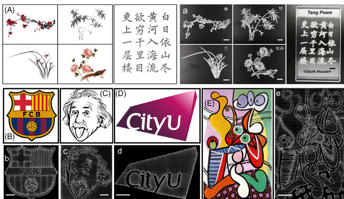
FIGURE 4 3D-printed PLA patterns. (A) Pictures of Chinese traditional paintings and an ancient poem. (B) Logo of the Barcelona football team. (C) Portrait of Einstein. (D) "CityU" logo of the City University of Hong Kong. (E) Painting by Pablo Picasso. (A–E) Corresponding printed patterns of (A–E). Scale bar: 1 cm.
