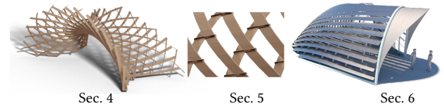
Fig. 4. Overview of applications. Gridshells formed by two or three families of rectifying strips are presented in Sec. 4 along with physical models. The difficult topic of gridshells with torsion-free nodes, where transversal strips meet at straight line segments, is addressed in Sec. 5. In Sec. 6 we design shading systems via a single family of rectifying strips.
