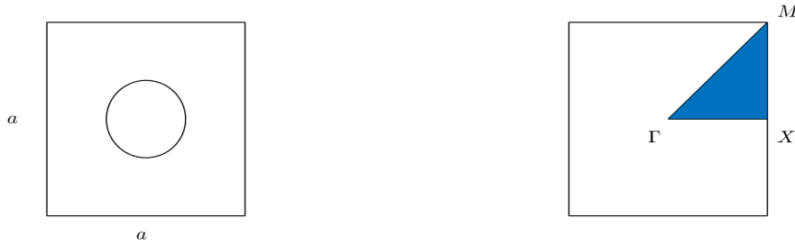
Figure 4: Square lattice: unit cell (left) and the corresponding first Brillouin zone (right). The IBZ is the blue area with vertices \Gamma = (0, 0) , X = \frac{1}{a}(\pi, 0) and M = \frac{1}{a}(\pi, \pi) .
