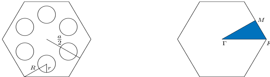
Figure 5: Hexagonal lattice: unit cell (left) and the corresponding first Brillouin zone (right). The IBZ is the blue area with vertices \Gamma = (0, 0) , K = \frac{1}{a}(\frac{4}{3}\pi, 0) and M = \frac{1}{a}(\pi, \frac{\sqrt{3}}{3}\pi) .
