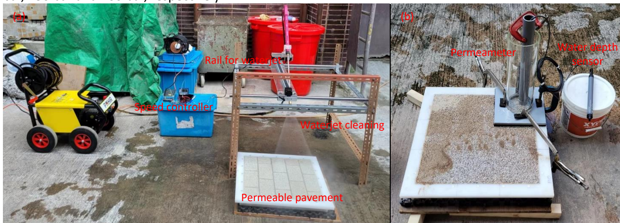
Figure 3. Pictures of (a) the waterjet cleansing on a permeable pavement trial slab in the laboratory (b) the circular permeameter for permeability test.
