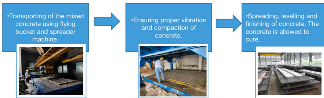
Fig. 3: Concreting and curing of a prefabricated RC slab.
