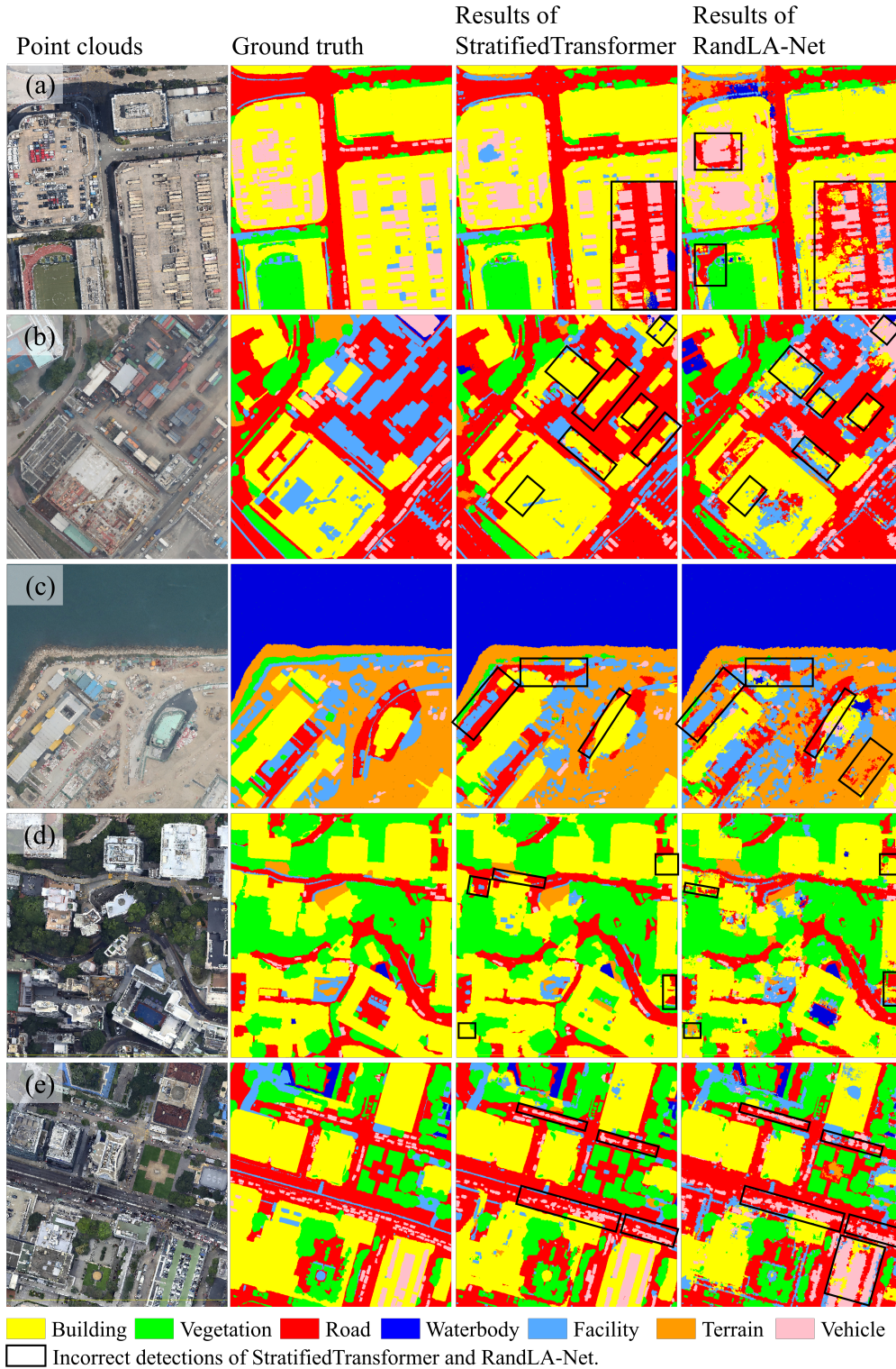
Figure 5: Typical errors of StratifiedTransformer and RandLA-Net on HRHD-HK. (a) Confusion between large-size building roofs and roads; (b)-(d) confusions between facility and building, roads and terrain, and roads and building podiums; (e) poor detection of vehicles.
