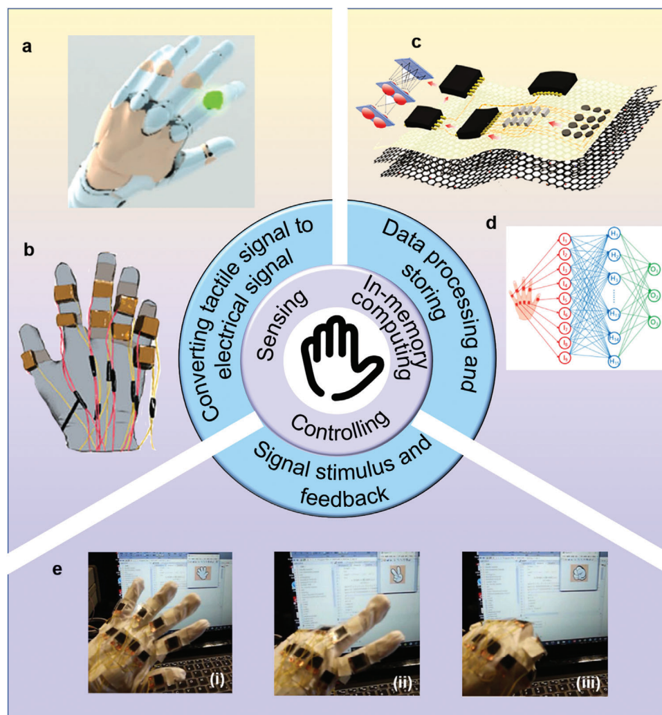
Figure 3. Schematic of sensing, processing, and controlling flow in tactile perception. a,b) Recent works on tactile sensing methods. Reproduced with permission. [25,26] Copyright 2022, Wiley. Copyright 2020, Wiley. c,e) Tactile signal processing algorithms and a complete tactile sensory system for object recognizing. Reproduced with permission. [27] Copyright 2019, IEEE Xplore.
