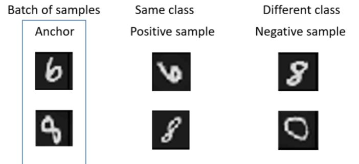
Fig. 2. Triplet generation: for one observational image \mathbf{x}_i with label \mathbf{y}_i , its positive set \mathcal{P}_i consists of images that are in the same class as \mathbf{y}_i , and its negative set \mathcal{N}_i consists of images that are with a class different from \mathbf{y}_i .
