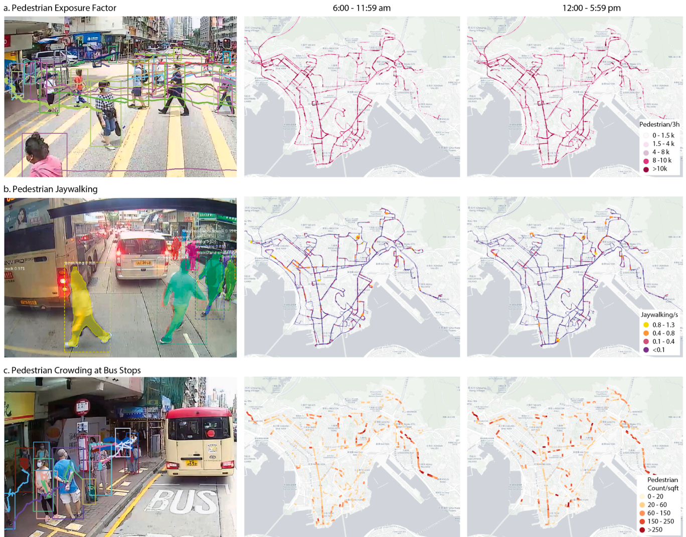
Fig. 2. Three behavioural risk factors constructed from the dashcam video. A) Pedestrian exposure. B) Pedestrian Jaywalking. C) Pedestrian crowding at bus stops. Maps of distribution are plotted accordingly at different times of a day.
