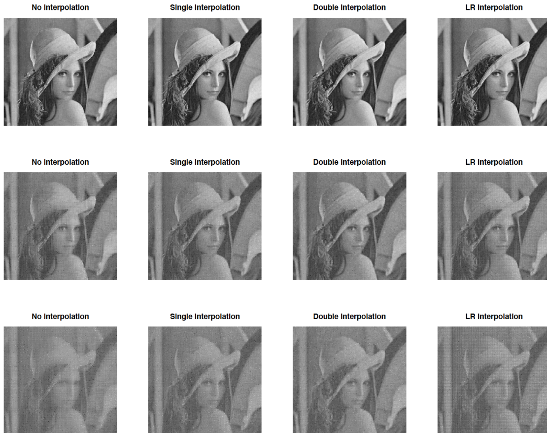
Figure 6: Recovered Lenna image with no interpolation (first column), single interpolation (second column), double interpolation (third column), LR interpolation (last column) when, \sigma = 0.05 (the first row), \sigma = 0.15 (the middle row), \sigma = 0.25 (the last row).
