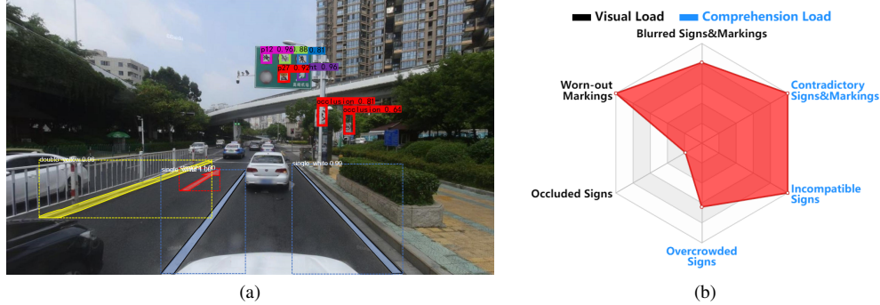
Fig. 10. A traffic violation hotspot caused by occluded signs and overcrowded signs. (a) The street view image of the scene with detection results. (b) The visual comprehension load profile.
