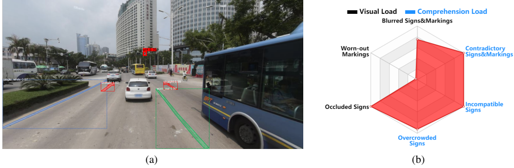
Fig. 9. A traffic violation hotspot caused by worn-out road markings. (a) The street view image of the scene with detection results. (b) The visual comprehension load profile.
