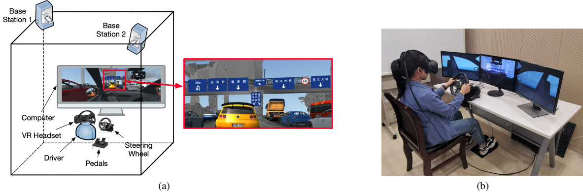
Fig. 1. The structures of the driving simulator. (a) An illustration of the driving simulator implement and a traffic scene with overcrowded signs. (b) The real-world deployment of the driving simulator.
