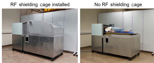
FIGURE 2 Experimental setups for quantitatively assessing the effectiveness of the proposed EMI elimination method in removing EMI-related image noise/artifacts for the 0.055 T MRI scanner. For comparison, a custom-made RF shielding cage (consisting of aluminum covers) was installed to fully enclose the subject, or was removed. EMI, electromagnetic interference; RF, radiofrequency.
