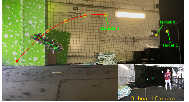
Fig. 1. Our quadrotor avoids a dynamic obstacle (a tennis ball), with relative speed up to 7.4 m/s. All perception, estimation, planning and control are performed by the onboard sensor (an Intel D455) and computer (a DJI Manifold 2 computer with Intel i7-8550U CPU). No prior knowledge of the size of the obstacle is required.
