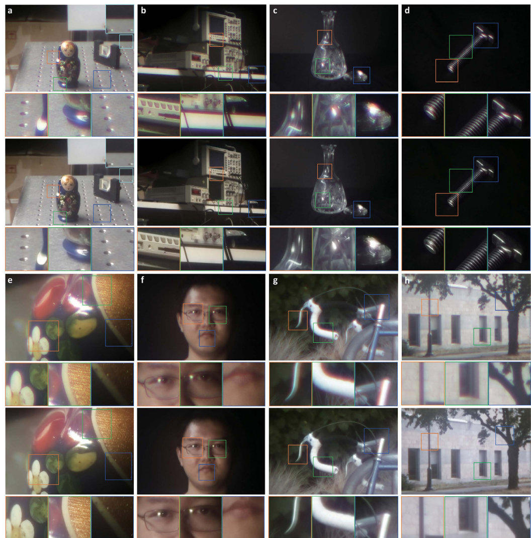
Figure 4. Results of static colour imaging with a single encoded lenses. For each individual result, both the blurry observation (top) and reconstruction (bottom) are shown for indoor and outdoor natural scenes. (a,b) Indoor scenes under fluorescent lamp illumination. (c) Transparent objects with reflective surfaces. (d,e) Small objects imaged in macro mode. (f) Human face. (g,h) Outdoor scenes under sunlight illumination. Insets in each result highlight the details before and after computational reconstruction. Chromatic aberrations are completely removed in all scenarios. The focal length range of the encoded lens for experimental results shown here is [100 mm, 300 mm].
