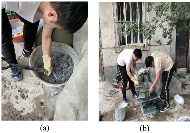
Figure 3: The process of casting concrete samples: (a) mixing concrete and (b) filling in the mold.
