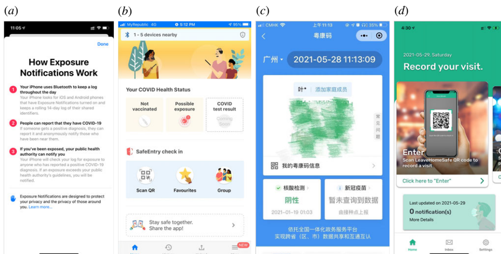
Figure 2. Three typical digital contact tracing apps: (a) Apple's Exposure Notification function (Bluetooth-based). (b) TraceTogether system in Singapore (Bluetooth-based). (c) Health Code system in Mainland China (Mandatory manual input), (d) LeaveHomeSafe system in Hong Kong (voluntary manual input). (Online version in colour.)
