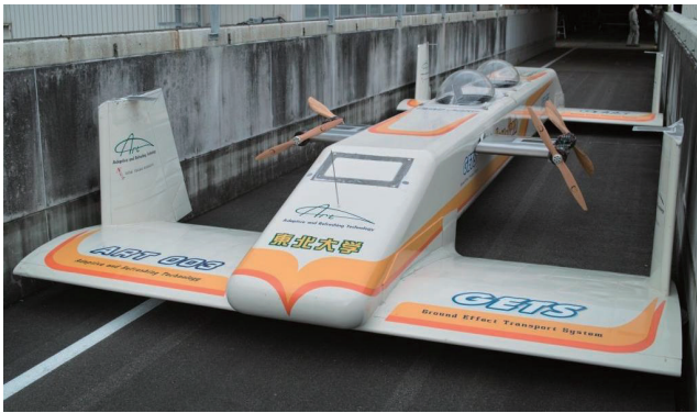
Fig. 20. Third prototype Aero-Train: manned experimental WIG vehicle ART003R.
