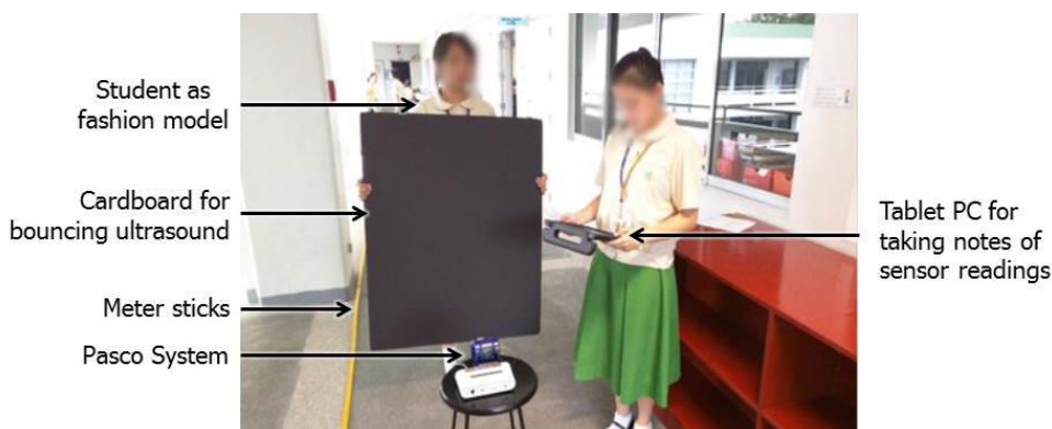
Figure 5: Two students from Miriam College High School perform the set of instructions for the fashion model scenario. A PASCO Motion Sensor is located in front of the student holding a black cardboard. Meter sticks are set on the floor to guide the student’s movement. A second student manages the sensor. She also collects the data from the sensor using a tablet computer.
