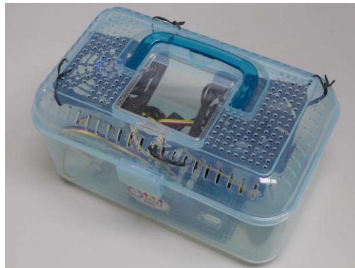
Figure 1. The present IEM could be stored in a hand-held box. Two fans are installed to maintain airy condition.
