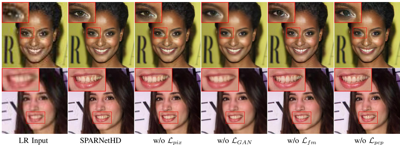
Fig. 12: Ablation study of losses used in SPARNetHD on the synthetic dataset CelebAHQ-Test (first row) and real dataset CelebA-TestN (second row). Better zoom in to see the details.
