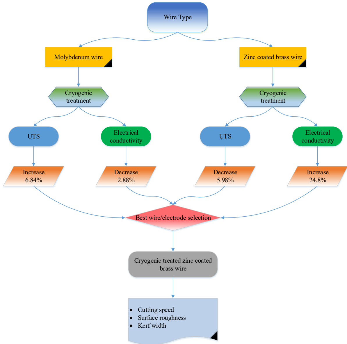
Figure 3. Framework for the selection of appropriate wire electrode for the machining of the squeeze casted Al2024/Al 2 O 3 /W hybrid composite
