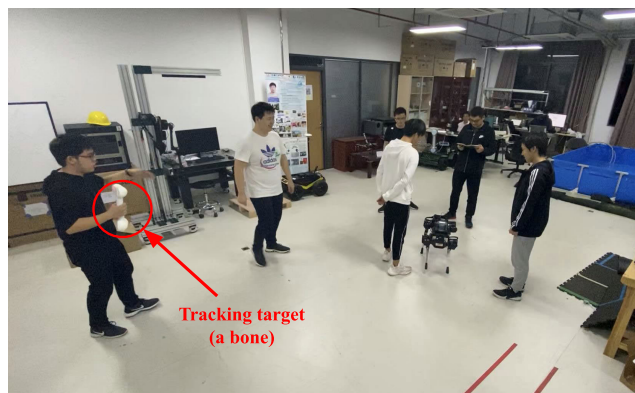
FIGURE 8. The demonstration of the dynamic collision avoidance experiments. We arranged 6 moving pedestrians in this scenarios about 4m x 4m in size.
