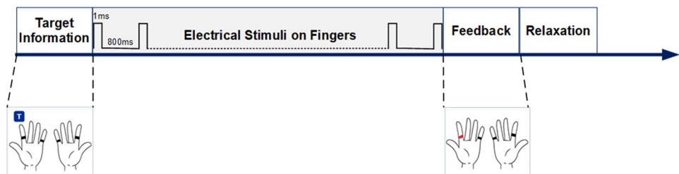
Fig. 2 Experiment protocol. Black band: Stimulation electrode position. Red band: Feedback of Stimulating electrode. T: the target position
