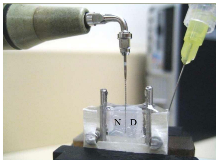
Figure 2. Experimental setup, with “N”= near-side to the ultrasonic handpiece, and “D”= distant side. Sterile saline solution was slowly injected into the simulated canal space to replenish any solution that was splashed out by the vibrating file.
