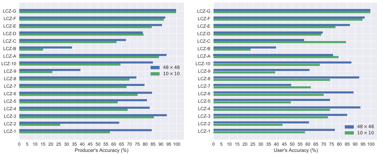
Figure 10: PA and UA obtained with 10 \times 10 and 48 \times 48 inputs.
