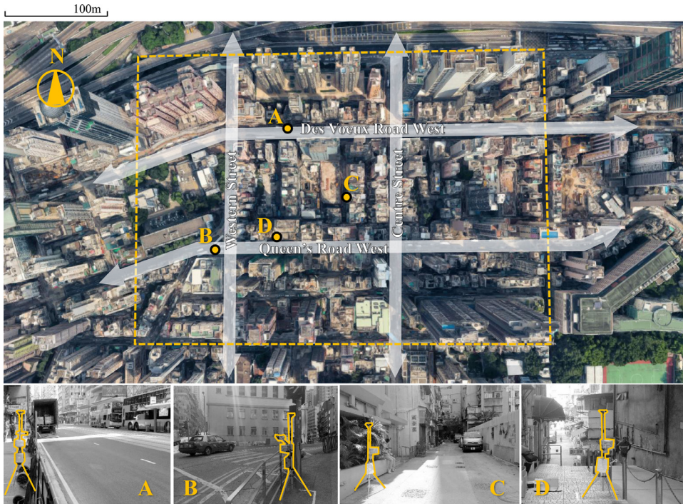
Fig. 4. (Upper) The Sai Ying Pun area of 252 m by 378 m and 4 measurement locations drawn on top of Google Earth imagery. (Lower) Site photos for the 4 locations with measurement equipment highlighted in yellow.
