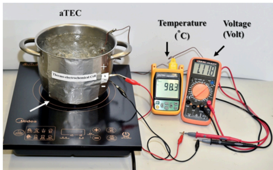
Figure 3: Demonstration of aTEC charged by a hot pot. Please click here to view a larger version of this figure.
