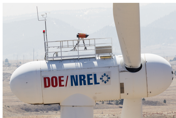
Figure 9. The pulsed LiDAR mounted on the three-bladed Controls Advanced Research Turbine located at the National Wind Technology Center in Boulder, Colorado [135]. Photo credit: Lee Jay Fingersh, National Renewable Energy Laboratory (NREL).
