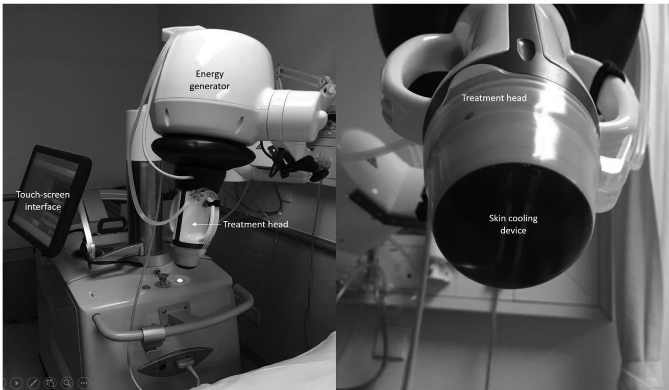
Figure 1. The ultrasound-guided high intensity focused ultrasound device for treatment of thyroid nodules.
