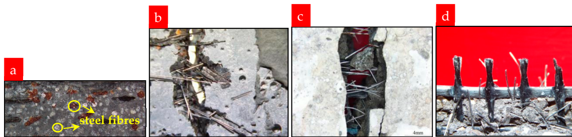
Figure 16. (a) Well-distributed steel fibers; bridging capacity of steel fibers in cracks: (b) P0C1S1, (c) P0C2S1; (d) fracture surface of TRM with steel fibers.
