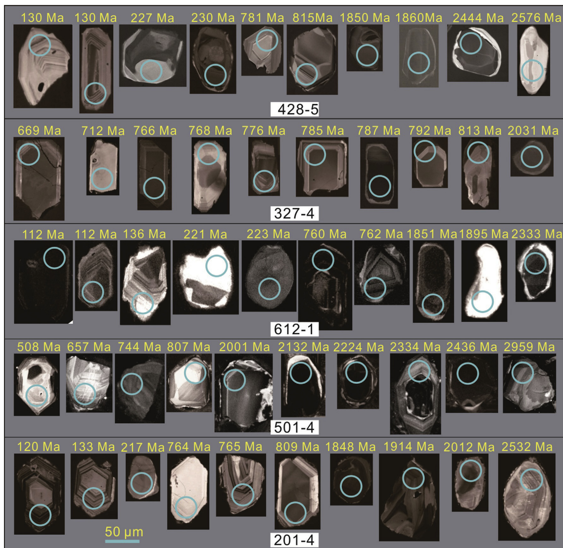
Fig. 4. CL images of typical detrital zircon grains analyzed in this study. The spot size of 30 \mu\text{m} corresponds to the laser beam diameter.
