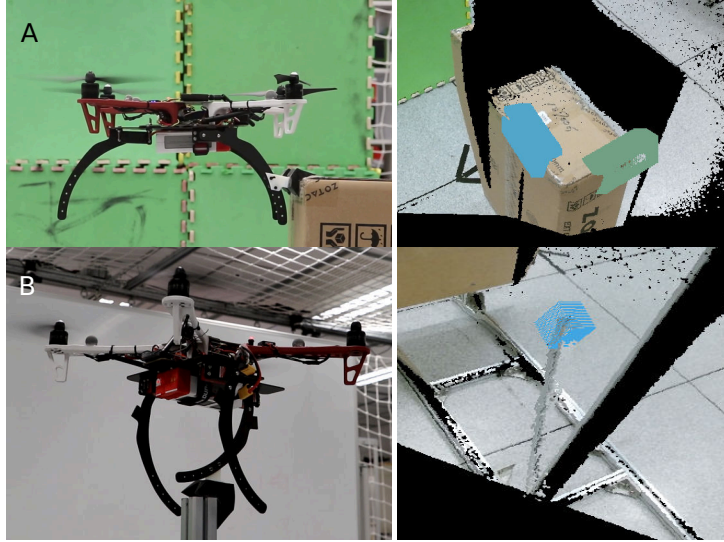
Figure 4: Example resting actions with vision-based perching and resting location detection: (A) Resting on a box's edge ( R_E ). (B) Stand-resting on a stick ( R_S ).
