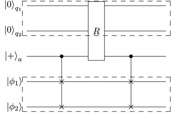
FIG. 2. Quantum circuit for implementing a modified exponential swap gate. An ancillary qubit is prepared at  $|+\rangle$ . Qumodes and qubits are not directly coupled.
