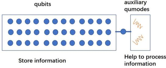
FIG. 1. Illustration of the hybrid approach that exploits the best of both qubits and qumodes. In our implementation of quantum linear regression, qubits and qumodes are minimally coupled by connecting only to an ancillary qubit.
