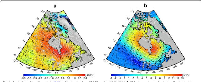
Fig. 1 Original data from Wang et al. (2015). a Gravity rates from GRACE models (2002–2014). b GPS-observed vertical velocities. The black dots indicate GPS stations
