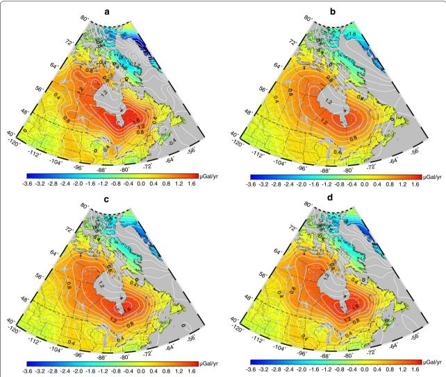
Fig. 8 The g-dot of real GRACE data and filtered results. **a** Original g-dot output; **b** filtered with 340 km averaging radius isotropic Gaussian filter; **c** filtered with 220 km averaging radius isotropic Gaussian filter; **d** filtered with 167 km averaging radius isotropic Gaussian filter
