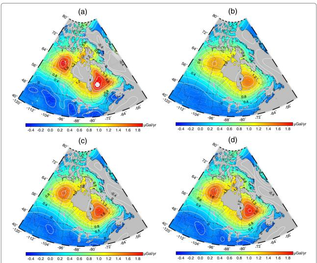
Fig. 7 ICE-6G\_C (VM5a) g-dot output and filtered results. **a** Original g-dot output; **b** filtered with 340 km averaging radius isotropic Gaussian filter; **c** filtered with 220 km averaging radius isotropic Gaussian filter; **d** filtered with 167 km averaging radius isotropic Gaussian filter
