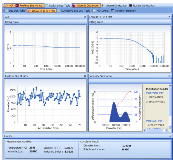
Figure 3. Particle size measurement of SDF-1 \alpha -DS-CS particles after freezing and thawing in water. In the absence of mannitol, the particles form aggregates after freezing and thawing. Note the formation of an additional intensity/size peak and the increase in cumulants diameter and polydispersity compared to that of Figure 1 .
