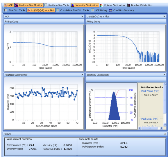
Figure 1. Analysis screen shot showing dynamic light scattering measurement of particle size. The top two panels show the plots of the autocorrelation function, G_2(t) , and logarithm of [G_2(t)-1] over time. The instrument's digital signal processor (correlator) expresses the detected light intensity as a function of delay time ( \tau ). The plot shows that SDF-1 \alpha -DS-CS particles caused an exponential decay of the intensity between 0.2-2 msec. To obtain the average decay constant \langle \Gamma \rangle , a program analyzes the \ln[G_2(t)-1] plot with cumulants fitting. The first order coefficient of the derived polynomial equation is assigned to \langle \Gamma \rangle , which is proportional to the slope of the curve. The second order coefficient divided by the square of \langle \Gamma \rangle is the polydispersity index, which describes the intensity distribution width. From \langle \Gamma \rangle the average diffusion coefficient ( \langle D \rangle ) and particle diameter ( d ) are calculated as: \Gamma = D \cdot q and D = k_B T / 3\pi\eta_0 d (Stoke-Einstein equation). The middle two panels show the fluctuation of the size reading during the 70 accumulation measurements, and the size distribution calculated with respect to intensity in the measurement. The cumulant diameter and polydispersity index are shown at the bottom of the screen.
