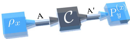
FIG. 1. Input-output test of a quantum device. To test the device \mathcal{C} , the verifier prepares an input state, randomly drawn from the set \{\rho_x\} . Upon receiving the input, the device generates an output, which is then measured by the verifier with the POVM \{P_y^{(x)}\} . The outcome is assigned a score and the average score is used as a measure of performance.
