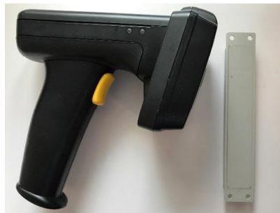
(b) Adopted UHF RFID reader and tag
