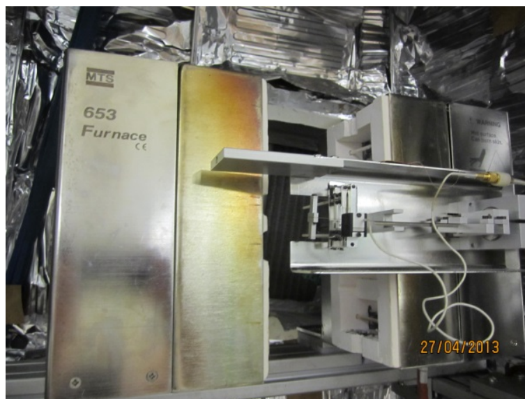
(a) Front view of furnace showing extensometer
