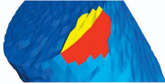
Fig. 4. Since normals in the red region have larger variations than those in the yellow region, DBSCAN is able to separate vertices in these regions into different clusters, and therefore, can achieve denoising without blurring the sharp edge between these regions.
