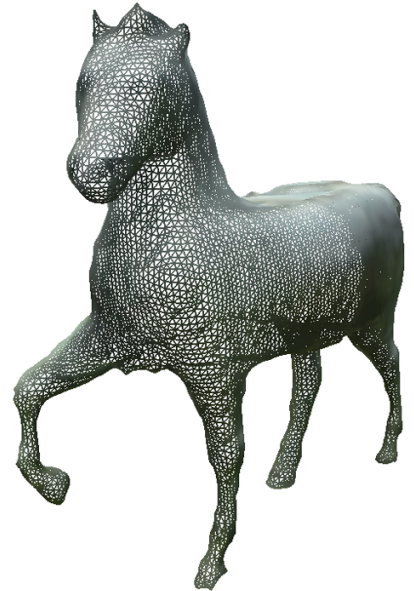
Fig. 9 Triangulated mesh of the 3D model built from the silhouettes and the estimated motion.
