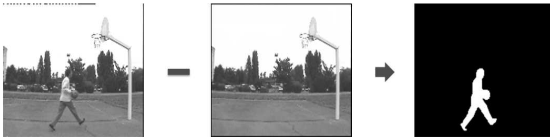
Fig. 1 Motion detection by background subtraction. Moving points are those where the current image and the reference image differ considerably.
