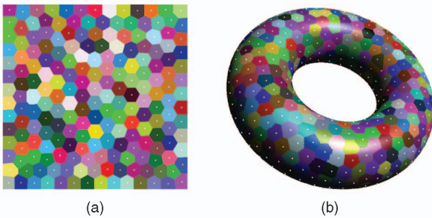
Fig. 1. (a) The CVT of a square 2D domain with 200 sites; (b) The constrained CVT on a torus with 600 sites.
