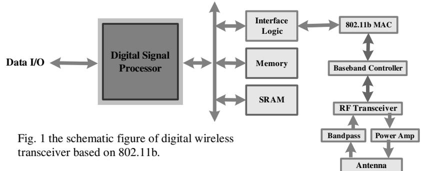
Fig. 1 the schematic figure of digital wireless transceiver based on 802.11b.
